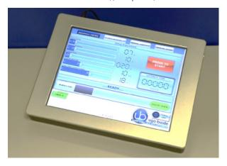
The "queen bee" is the 40500-001 Touch-Screen Controller, a powerful tool incorporating a 12" touch-screen, which will function as main unit in a number of tests, via the dedicated application software:
