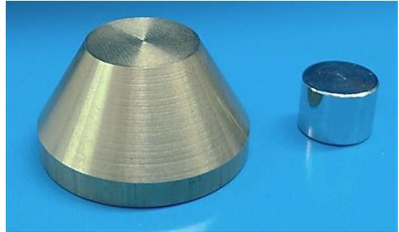
You can find both weights in the accessory case. If you select the 5g weight, start the calibration by depressing the **F2 (5g)** key. At the end of the procedure, confirm by the **F4 (OK)** key.
