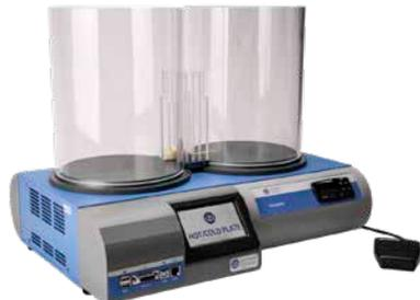
Thermal Place Preference (TPP Test) for Mice & Rats
