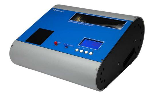
Ugo Basile Blood Pressure Recorder is a reliable pressure generator that provides smooth and stepless pressure build-up.
