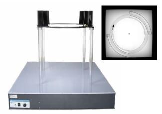
IR Eleveted Zero maze and LUX IR Illuminator, with infrared view from the video-tracking software
