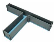
T-Maze with mat plastic walls and opaque metal floor
