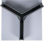
Y-maze with IR transparent walls and floor on LUX IR Illuminator
