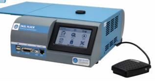
mal feels pain and flicks its tail, a sensor detects it, stops the reaction time counter and switches off the bulb. The reaction time of the animal is thus automatically determined to the nearest 0.1 second. Mice holders available.
