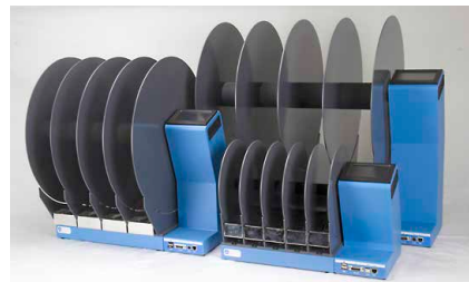
Rodent Treadmill NG with interchangeable lane assembly for rats or mice
