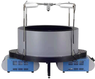
TGR - Thermal Gradient Ring (Zimmermann's method)
