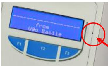
If the problem remains, charge the internal battery and reset the e-VF manually by pressing with a needle into the small reset hole located to the right of the display.
