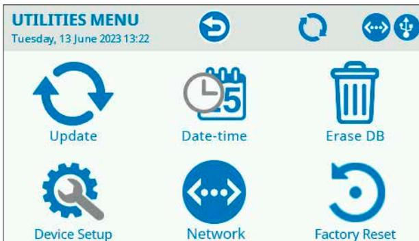
The **UPDATE** menu requires to insert the USB pen drive and is necessary to update the device firmware. Contact the Ugo Basile Support team before updating the firmware, providing the device serial number.
