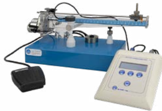
37215 - Analgesy-Meter Randall-Selitto paw-pressure test
