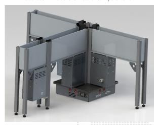
An automated door is provided on each arm, at the central arena end; the "start" compartment with automated door, attached to the end of the stem-arm, completes the T-Maze.
