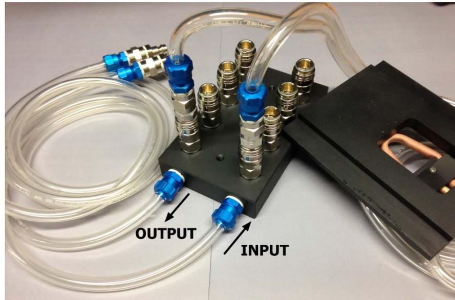
After connecting the tube to the mechanical stimulator, fix them into the brackets provided, as shown on the picture on the right.
