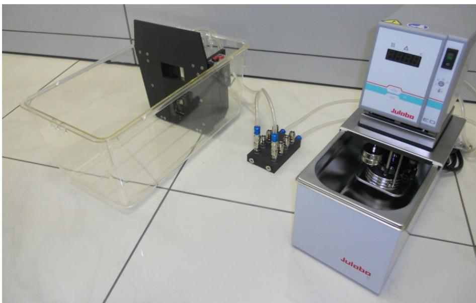
Setting-up a Standard System consists in assembling the stimulation wall, connecting all the parts electrically and hydraulically, and installing the software. The pictures in the following paragraph will guide you through the process.
