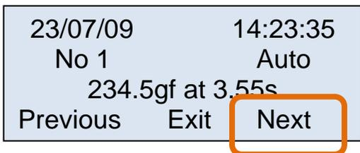
The most relevant information of each measurement (Date, Time, Progressive number of the measurement, Automatic or Foot Pedal measurement mode, Peak Force, Peak Time) are shown and the measurements can be browsed by simply pressing **Next**.
