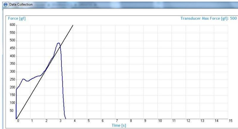
The experimenter can consistently apply the force at the desired rate, by simply making sure that the blue trace lays on the black line.
