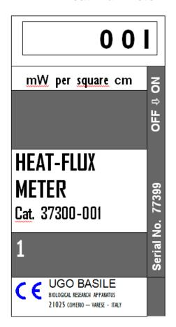
The Meter upper panel features a 3-digit display which indicates the heat-flux, whose measuring unit (mW per square cm) is indicated below the display window.
