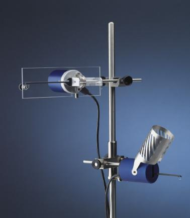
The picture shows an **Isotonic** Transducer (left) & an **Isometric** Transducer (right), see separate datasheet
