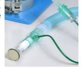
The picture shows a mouse nose-cone/mask, connected to an evacuation tubing.
